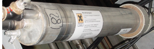
Figure 1: 100-kW, 500-MHz coaxial load for 30% glycol-water coolant. The load type was designed and build at DESY. Due to the usage of glycol the attenuation constant has been increased from about 17dB/m to 26dB/m @ 30°C coolant temperature. Thus it was feasible to make the design relative compact.
