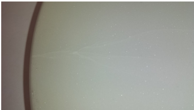
Fig. 9: On the untreated side of the window hairline cracks were visible.
