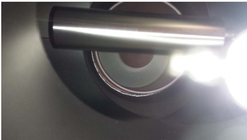
Fig. 14: 7 th evaporation attempt. Vacuum window of the coupler S/N 65-83 after Ti coating. The photo was taken through the quartz window after 45 seconds sublimation time at 55.5 A filament current
