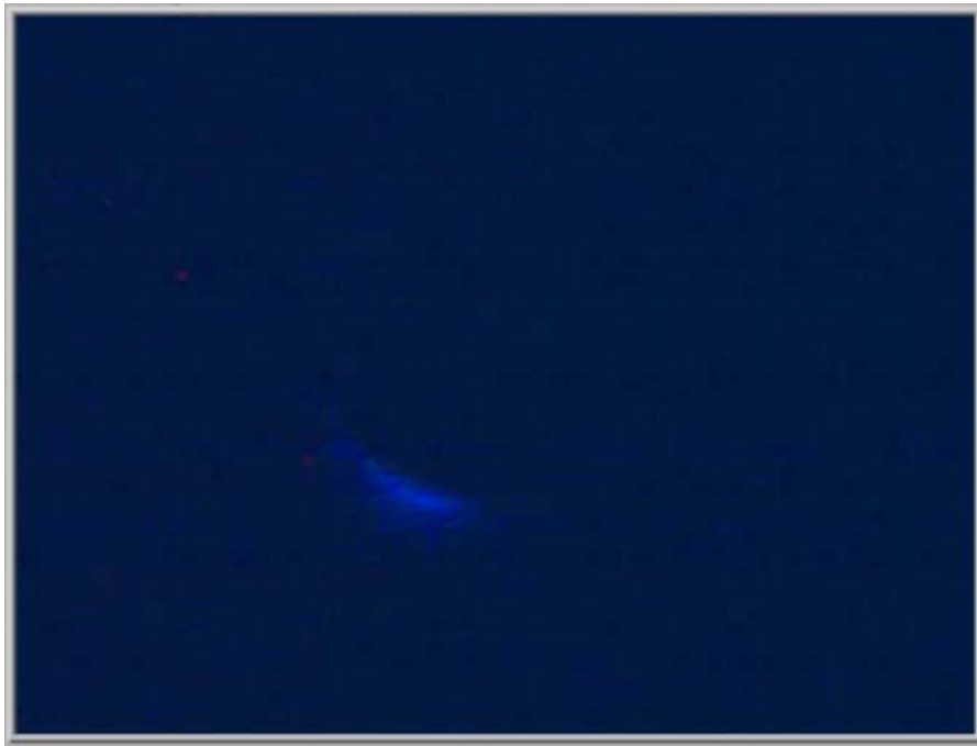
Fig. 15: Slight bluish glow of the Ti coated coupler S/N 65-83 during the conditioning process at 230 kW RF power and 1.1 \cdot 10^{-8} hPa vacuum pressure
