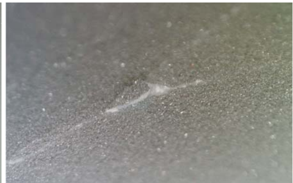
Fig. 10: On the coated side of the window, a tiny, millimeter-sized piece was broken out.
