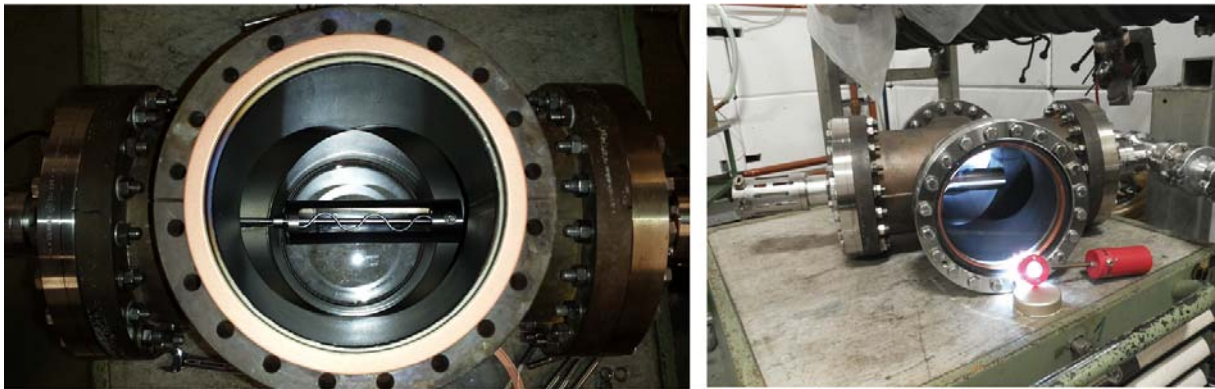
Fig. 3: Vacuum cross-chamber with the VARIAN Ti Sublimation Cartridge inserted
