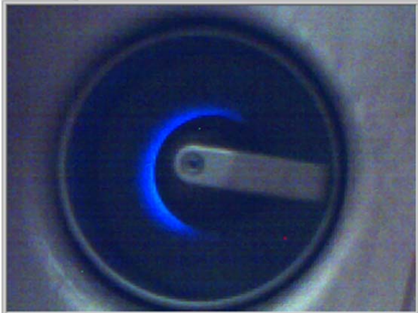
Bluish glow of the titanium coated coupler window at the beginning of the conditioning process at 50 kW RF power and 10^{-7} hPa vacuum pressure
