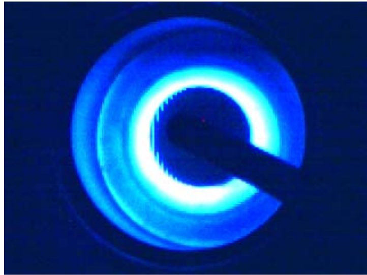
Fig. 11: Coupler S/N 014-82 before titanium coating at 190 kW RF power and 5 \cdot 10^{-8} hPa vacuum pressure
